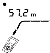
Figure 6.15 Open on Coaxial Cabling
