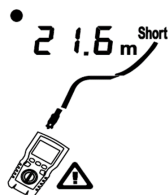
Figure 6.16 Short on Coaxial Cabling
