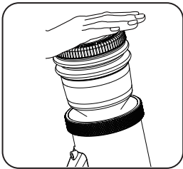
Step 3 Place your hand above the bean cup cover, gently press the bean cup cover, and blow the residual coffee powder out of the machine.
