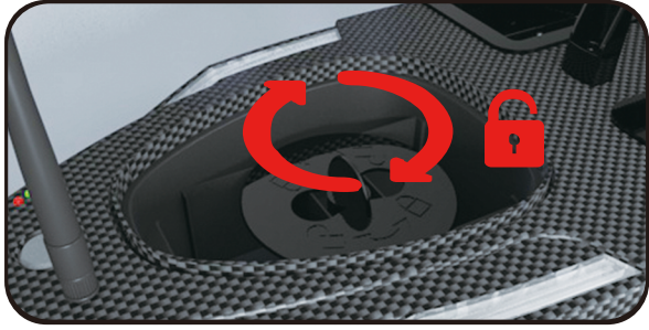
Take Out The Battery And Install Turn clockwise to open and remove the battery, press the holder into place and turn counterclockwise to secure
