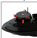
② Unscrew the nut and remove the battery compartment cover
